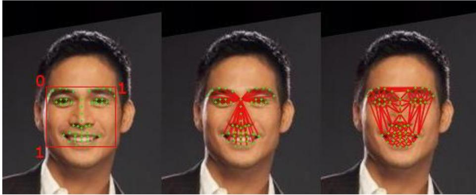
Fig. 1. Illustration of geometric feature vectors considered in our work. *Left*: Normalized landmark coordinates. *Middle*: Angles/distances between landmarks. *Right*: Triangle areas.
