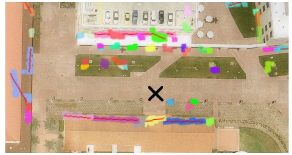
Figure 5: An aerial view of the group and planar information for the data set from Figure 1. Each range point is represented as a dot, and color represents groups. Extracted planes are represented as red lines. The user collected the data set from the black X location. Note that the aerial photograph is not ortho-rectified. Groups not on building surfaces are due to entryways, trees, or lamp poles.
