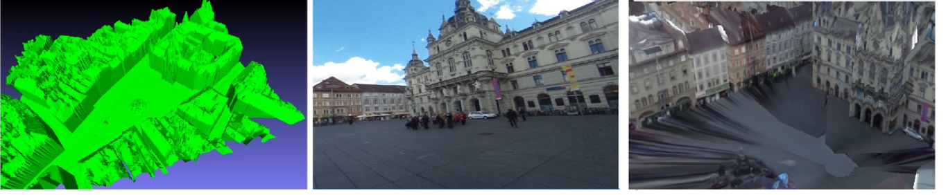
Figure 1: The system uses a geo-registered mesh model (left) and panorama images (middle) as input. Using projective texture mapping, both input data sources are combined to produce virtual renderings of the environment (right).
